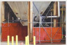
Thermal Resistance -70°F to 800°F 800°F for polymer covering (2 minutes) 2525°F: Maximum temperature tested by A.R.C. 7320-R was developed to provide an excellent performance, economical welding fabric for protection of personnel and equipment during welding operations. A user-friendly product, the 7320-R is a welder's best friend!
