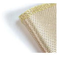
These products are part of a family of flexible silica textiles with excellent break strength and improved abrasion resistance.
