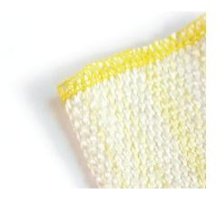
2240HT Textile is woven from continuous "E" glass. Totally free from any asbestos.
