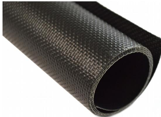
Three high strength plies of PTFE film were laminated to produce the barrier. The resulting 0.009 in. (0.23 mm) thick PTFE barrier is durable, flexible, and stress crack resistant.
